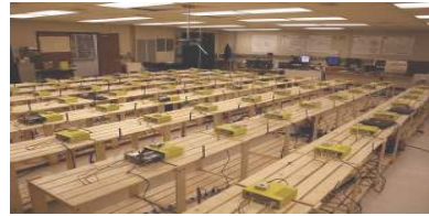
Fig. 1. The prototype ORBIT indoor testbed comprises 64 nodes (small form factor PCs) arranged on a grid.
