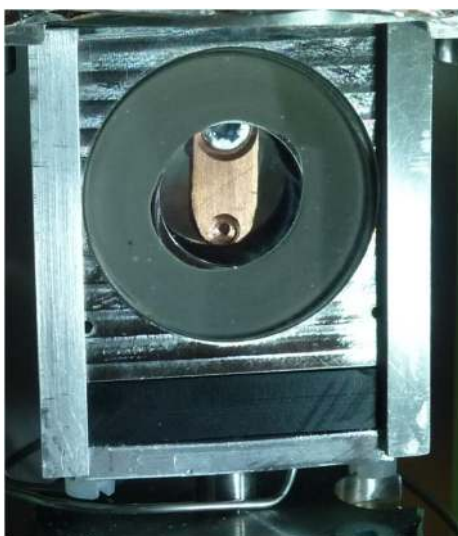
FIG. 8. The target frame is shown here as seen from the frontview camera (but with a larger field of view to illustrate the surroundings). With the glass windows (quartz in the picture, later changed to sapphire for greater durability), the target is visible even with the growth chamber closed.
