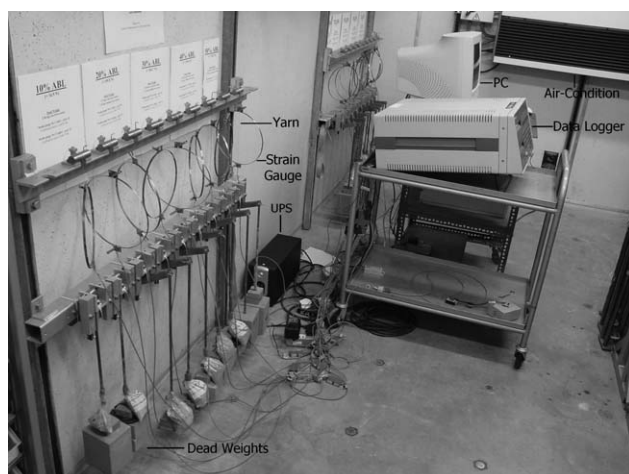
Figure 6 Experimental set-up for CCT tests.
