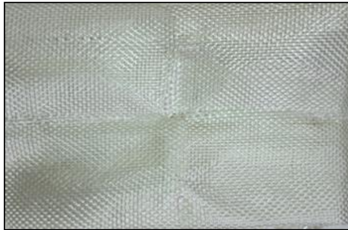
Figure (12): - Fiber glass type (E-glass) woven rove with angle of (0-90) continuous direction with surface density (0.5 Kg/m 2 ).
