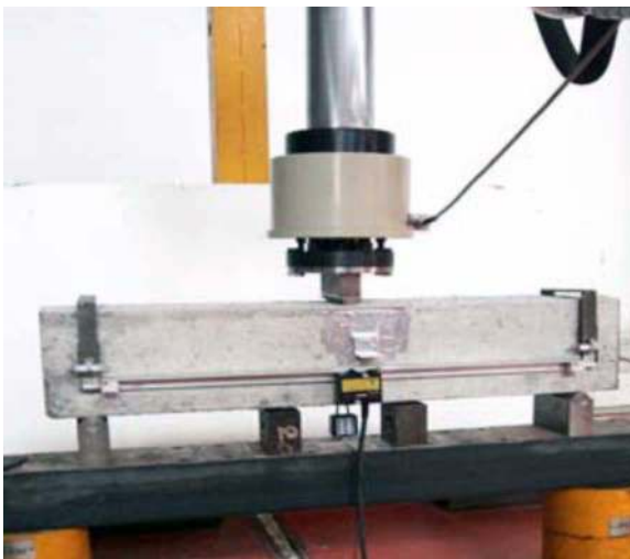
Fig. 2. General view of experimental fracture test setup
