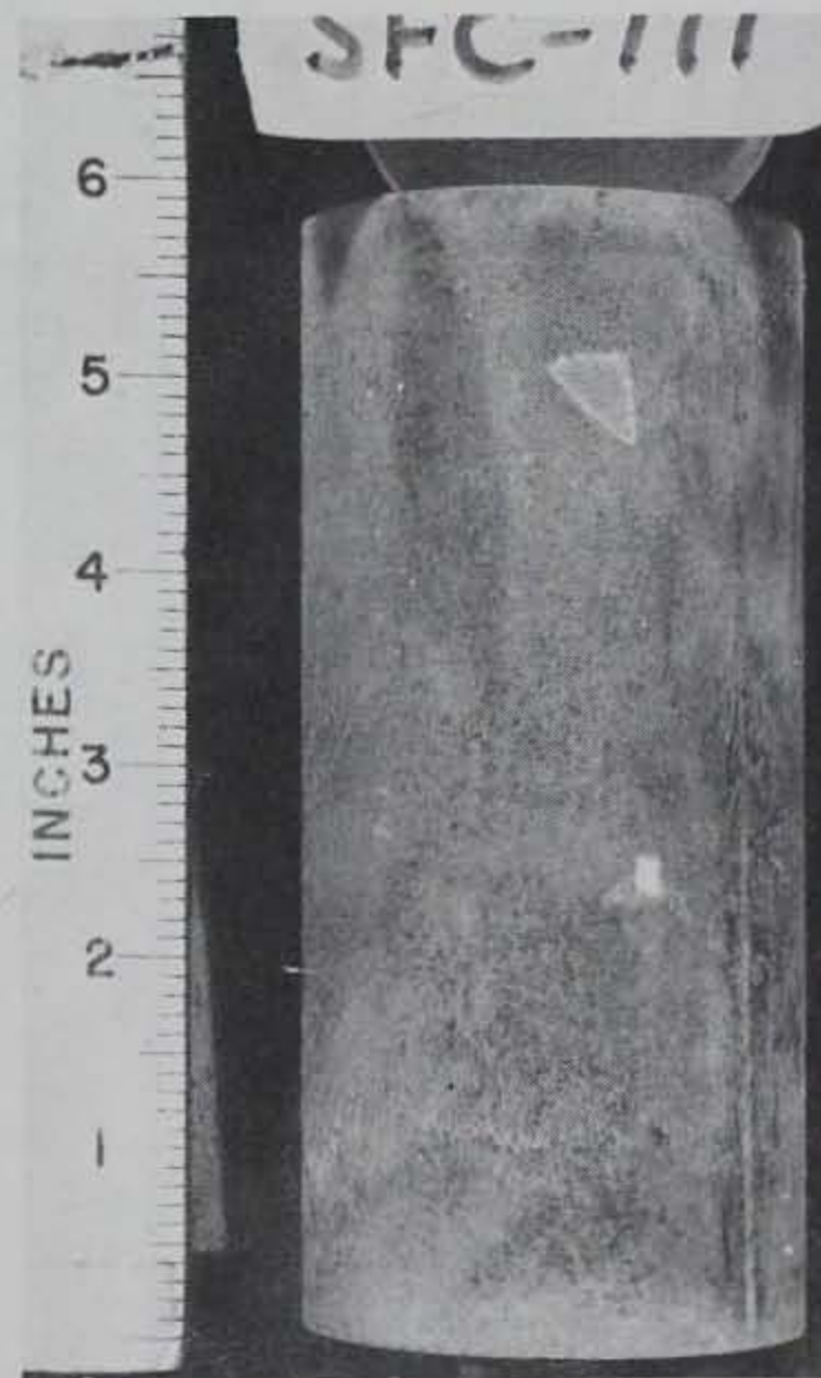
d. Suffield clay specimen subjected to 140 psi (20% of instantaneous strength) for 750 hr at 15^{\circ}\text{F} , e = 1.06 .
