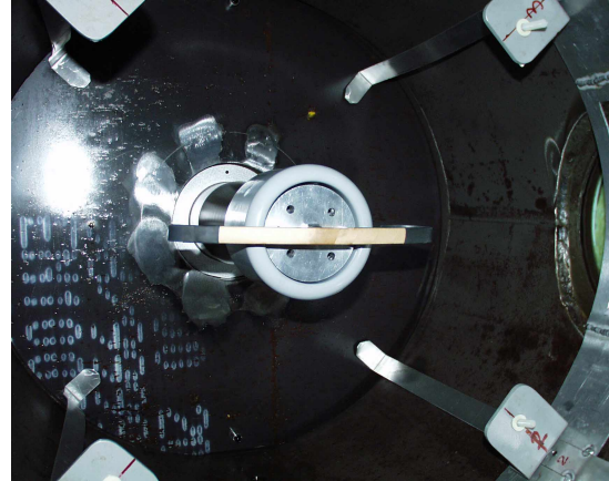
Fig.2. Internal view of test cell showing electrode and carrier on bushing
