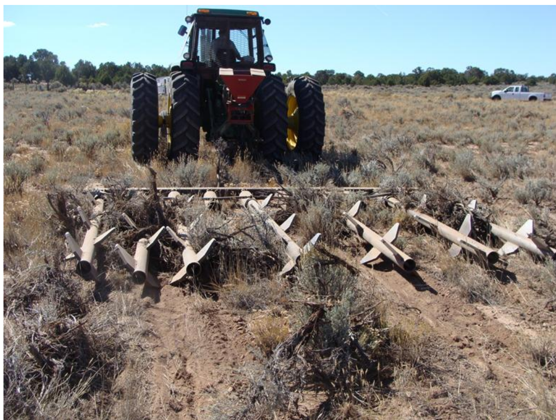
Figure 1. Photo of a dixie harrow. Toothed metal pipes are dragged behind a tractor. This can remove some of the shrubby overstory and thin out understory plants (grasses and forbs). Desirable seeds are spread in front of the tractor so that they are incorporated into the soil as the harrow passes over them (Photograph by J. Dollerschell).
