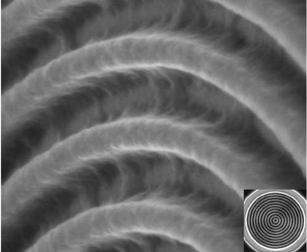
Fig. 10. Tilted view of a radial grating feature, along with a top-down view for reference, demonstrating the importance of the substrate interface in the LER.
