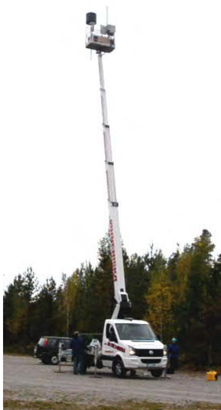
FIGURE 6. Rapid network deployment with crane cars.
