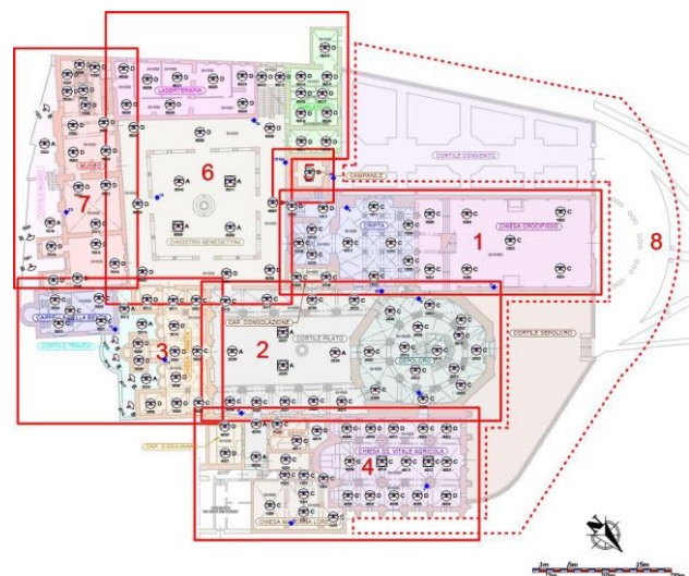
Figure 3. Map of the scanning positions during the survey of St. Stefano Basilica. In order to ensure greater readability, the map shows only some of the performed scanning locations and in particular those relating to the ground floor.
