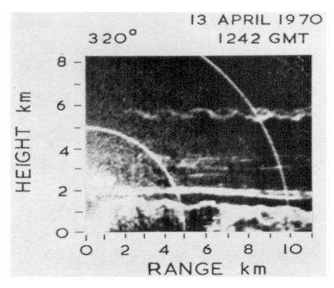
Figure 3: Radar observation of a Kelvin-Helmholtz billow at 5.6 km altitude.
