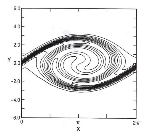
Figure 4: Pseudospectral simulation of a Kelvin-Helmholtz billow with  $J_0 = 0.10$  and Re = 200; the contours shown are isopycnics (i.e., constant-density contours).
