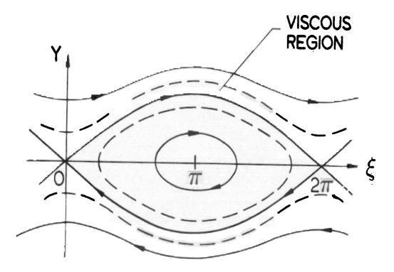
Figure 2: Streamline pattern in the nonlinear critical layer.
