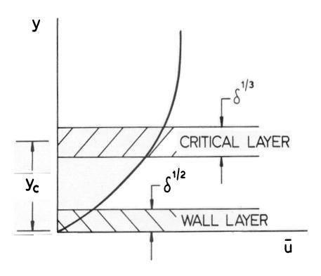
Figure 1: Boundary layer profile showing location of viscous layers.
