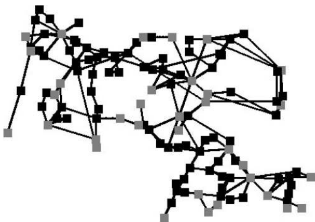
FIG. 2. Diagram of the IEEE 118 bus network. Generators are gray squares and loads are the black squares.
