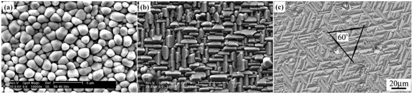
Figure 16 : (a) Top-view scanning electron microscopy SEM image of \text{Cu}_6\text{Sn}_5 scallop-type grains on a \text{Cu} [128]; (b) Morphology of rooftop-type \text{Cu}_6\text{Sn}_5 formed on (100) \text{Cu} [128]; (c) on (111) \text{Cu} [129].
