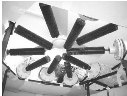
Fig. 8: An arrangement of the heat pipe/PCM units below a ceiling fan proposed by Turnpenny et al. [178].
