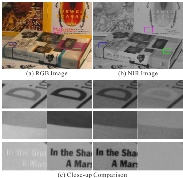
Figure 1. Appearance comparison of RGB and NIR images. (a) RGB image. (b) Corresponding NIR image. (c) Close-ups. The four columns are for the R, G, B, and NIR channels respectively.
