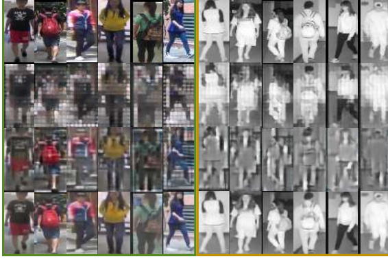
Figure 3. Reconstruction examples. The 1 st to 4 th rows correspond to original images, shared feature reconstructions, specific reconstructions and all feature reconstruction results, respectively.
