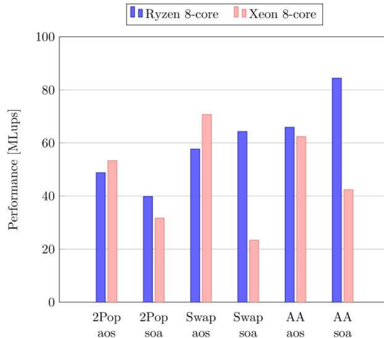
Fig 3. Performance of CPUs with a modest core count. All simulations are executed with the BGK-W2 collision model and N = 128 . On both CPUs, best performance was quite unpredictably obtained sometimes with and sometimes without loop unrolling. The plotted value shows therefore always the best of the two.
