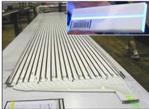
Figure 23: Photograph of a single scintillator strip containing a WLS fibre along with a photograph of a collection of strips mounted side-by-side in a module. The WLS fibres are collected by the manifold at the bottom of the picture to be routed out to the optical connector. Photographs courtesy of [50].
