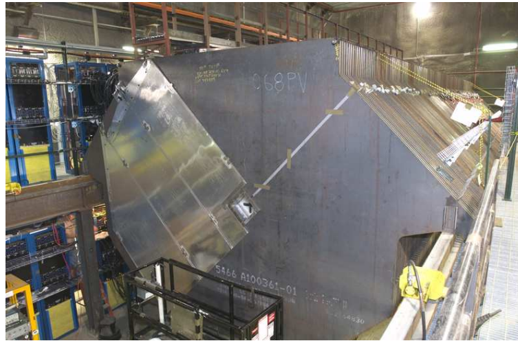
Figure 26: Photograph of the Near detector during installation. The coil hole can be seen along with an aluminium-covered scintillator module, the module does not extend the entire length of the steel as this is a partially-instrumented plane. The racks on the right-hand side run along one side of the detector and hold the PMTs and readout electronics. Photograph courtesy of [50].
