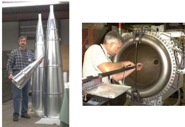
Figure 20: Photographs of the NuMI parabolic focussing horn inner conductors (left) and bottom-view (right). Photographs courtesy of [50].
