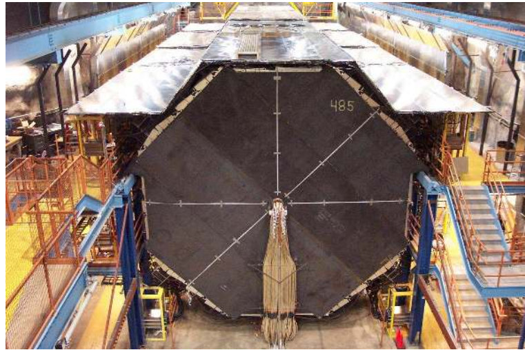
Figure 25: Photograph of the Far detector. The magnetic coils can be seen entering the centre of the first 8 m diameter octagonal plane. The PMTs and readout electronics are situated at the left- and right-hand sides of the detector along the walkways. The cosmic ray veto shield can be seen above the detector. Photograph courtesy of [50].
