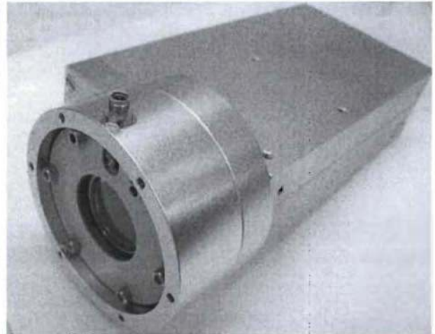
Figure 6. 18 mm cross strip sealed tube mounted in a housing with a preamplifier board enclosure attached behind.
