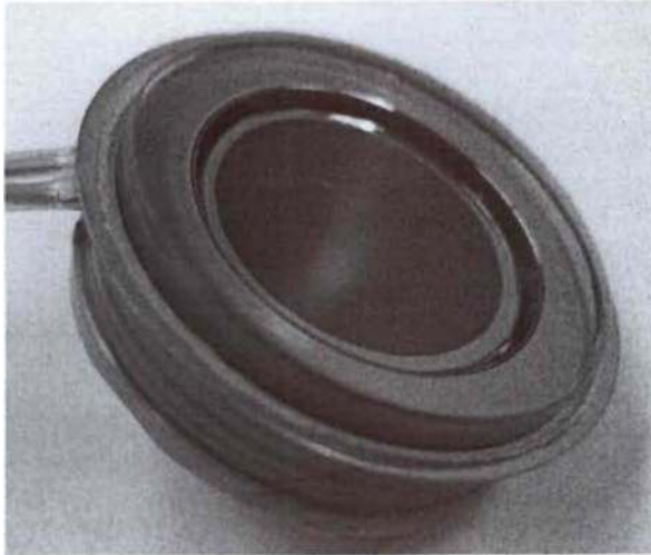
Figure 3. 18 mm sealed tube MCP detector with a 22 mm cross strip anode and a SuperGenII photocathode on the input window.
