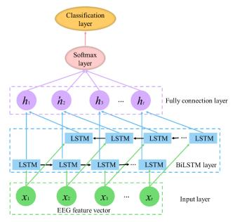
**Figure 4.** BiLSTM network architecture. It consists of five layers (input layer, BiLSTM layer, fully connection layer, softmax layer, and classification layer).  $x_t$  is the EEG feature of time t.  $h_t$  is the hidden state of LSTM cell in time t.
