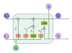
**Figure 5.** The details of a LSTM memory cell. It contains two kinds of activation functions ( $\sigma$  and tanh).  $C_t$  is the LSTM cell state in time t.  $f_t$ ,  $i_t$ , and  $o_t$  represent the outputs of forget gate, input gate, and output gate in time t separately.
