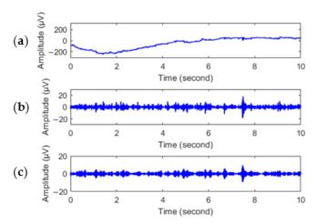
**Figure 3.** EEG signal preprocessing; the units are  $\mu V$ . (a) The original EEG signal; (b) the gamma wave obtained by wavelet decomposition; (c) the gamma wave after artifact removal.
