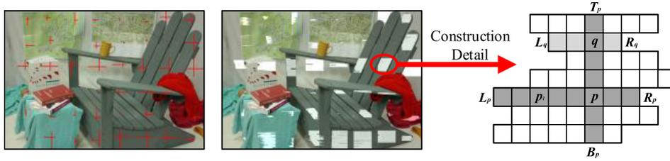
**FIGURE 2.** The left part shows cross skeletons with randomly selected anchor pixels as the centers. The white regions in the middle image are constructed cross patches. The right image shows one cross patch construction detail: the cross patch is made up of the union of horizontal arms ( $L_q$  and  $R_q$ ), whose center pixel  $q$  is on the vertical arms ( $T_p$  and  $B_p$ ) of pixel  $p$ .
