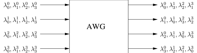
Fig. 1. Considered routing for the AWG device.
