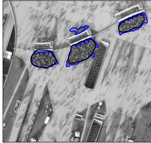
Fig. 4. Detected crowd boundaries using the first-order statistics. The detected crowd boundaries are represented in black. The ground truth for crowd boundaries is represented in blue.
