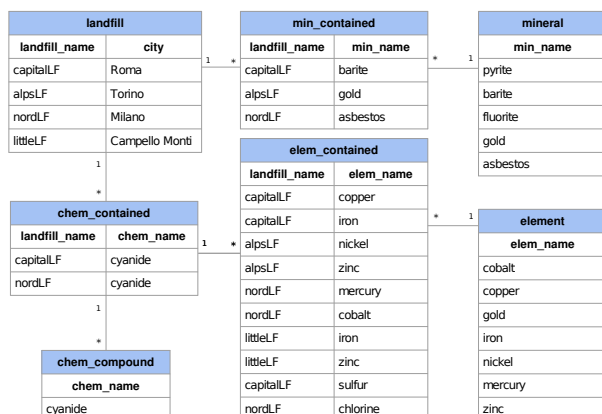
Fig. 1 Sample fragment of the SmartGround database: this segment of the database represents a sample data fragment capturing the knowledge of what is contained (in basic terms of elements, minerals and chemical compounds ) in four mine landfills
