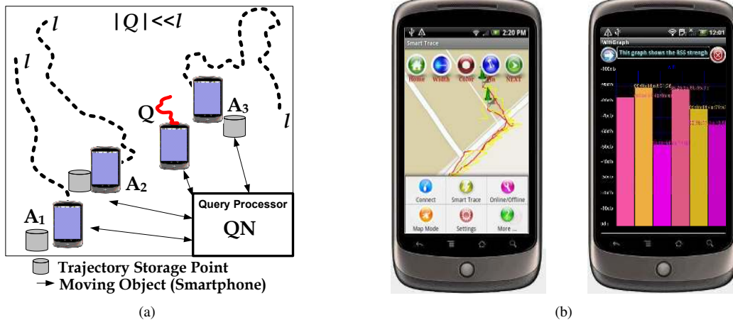
Fig. 2. SmartTrace + [9]: The SmartTrace + project enables trace similarity search among smartphone users. It answers queries of the form “Report the users that move similar to Q ”, where Q is some query trace. It optimizes such queries with respect to response time and energy consumption on the smartphones, without sharing the personal trajectories with the query processor. (a) Our system model. (b) Screenshots of the SmartTrace + client for outdoor environments with GPS and indoor environments with RSS signals.
