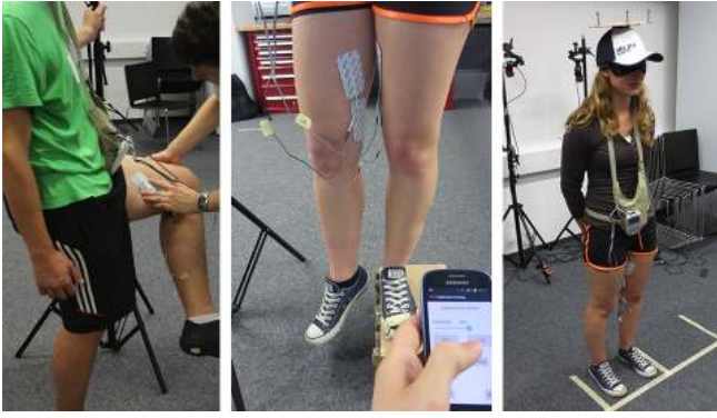
Figure 5. Placing the pads on the musculus sartorius (left) and measuring the angle of deflection corresponding to EMS intensity (right).
