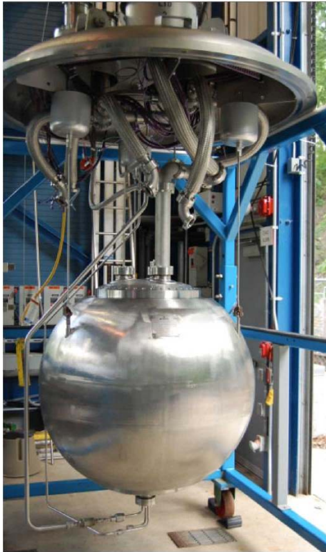
Figure 3.—Altair LDAC-1 flight representative test tank integrated with SMiRF vacuum chamber lid.
