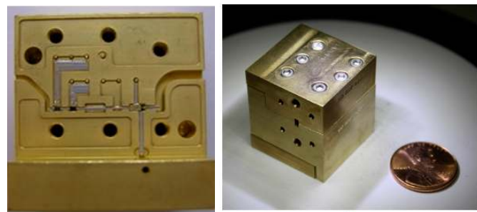
Fig. 4. Multi-chip MMIC Module for G-Band, split-block view at left, and fully assembled module with penny for scale at right.
