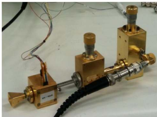
Fig. 9. Photo of the G-Band receiver module, with local oscillator applied at room temperature.
