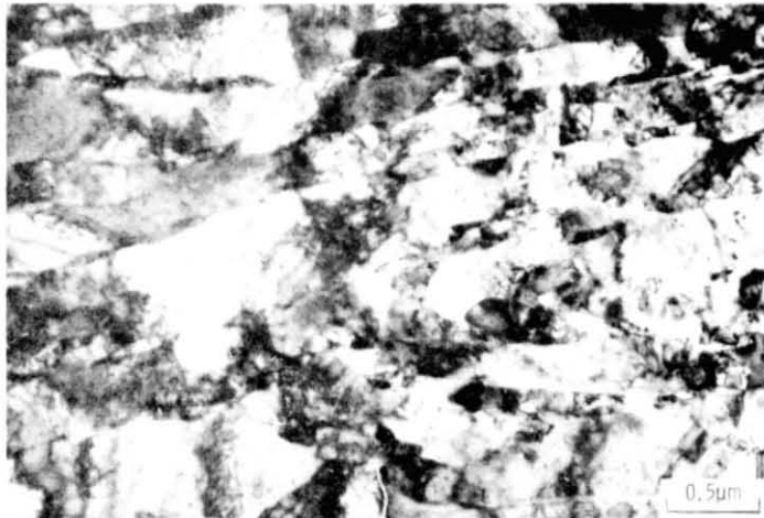
Figure 7. - Transmission electron micrograph of Fe-12Ni-0.5Al-2Cu alloy illustrating bowing of dislocation around less than 400 Å diameter Cu precipitates.
