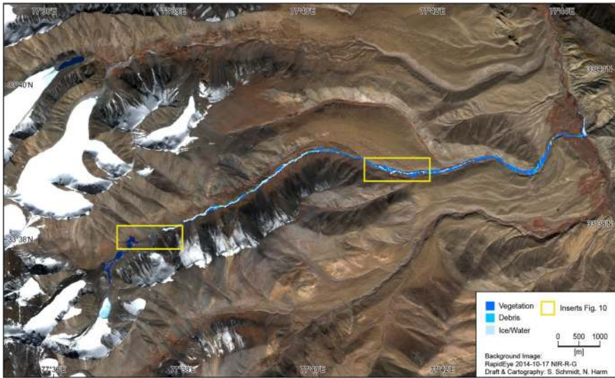
Fig. 11 Gya valley with reconstruction of the GLOF—the conducted change detection analysis shows the flooded area classified into three cover type dynamics: vegetation to debris, modified debris and ice-covered to debris-covered area
