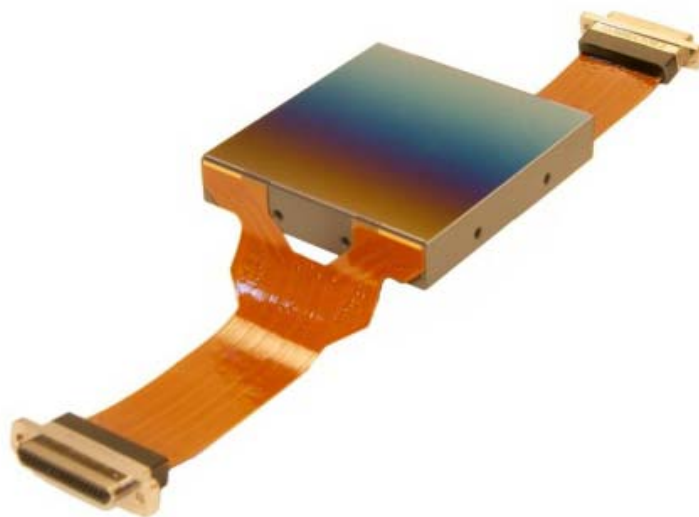
Figure 2. The CCD231-84 detector showing the two low-thermal-conductivity flex ribbons.
