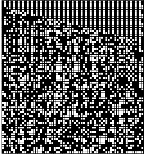
Fig. 10: Round keys (one per row) using master key (1010 \dots 10 \parallel 1010 \dots 10) for Simon128/128. A black square represents a 1, a white square 0.
