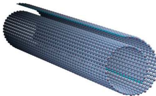
Fig. 5 A portion (45 unit cells are pictured) of the one-dimensionally periodic rolled nano-scroll used in the benchmark calculations of the parallelized CRYSOR program.
