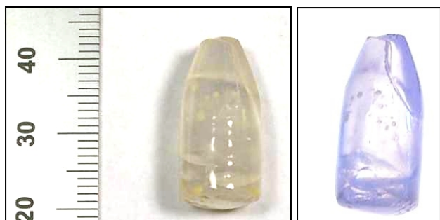
Fig. 1. Photograph of a \text{SrI}_2:8\% \text{Eu} ingot. The photograph on the left was taken with ambient light, while the photograph on the right was taken with the ingot placed on a light box.
