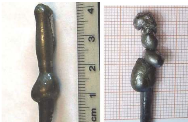
Fig. 2. Samples resulting from crystal growth experiments from the stoichiometric melt with upper and lower rod rotation. Left - Successfully grown single crystal ( sc1 ); Right - The crystallized ingot experienced repeated dropping down of the melt because of the unfavorable combination of the high density and of the low surface tension of the melt.
