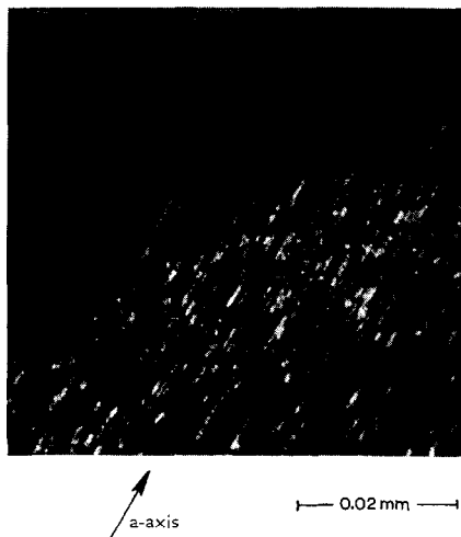
Fig. 5. Surface of a cleaved lead bromide crystal irradiated by a high pressure mercury lamp (Philips H.P.K. 125) for 30 minutes through a grid of an electron microscope. A small part of the shadow of this grid can be seen where the crystal was not irradiated. Optical microscope: Reichert Zetopan with interference contrast technique according to Nomarski.
