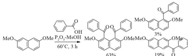
Scheme 1. Synthetic reaction of the title compound: P_2O_5 -MsOH mediated direct condensation of 2,7-dimethoxynaphthalene with benzoic acid.
