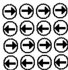
Fig. 13. Ordering of the atomic dipoles in an antiferromagnetic material.
