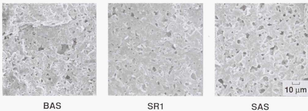
Figure 8.—SEM micrographs of fracture surfaces of different glass powder bars sintered at 1500 °C for 20 hr. The micron marker shown applies to all the three micrographs.
