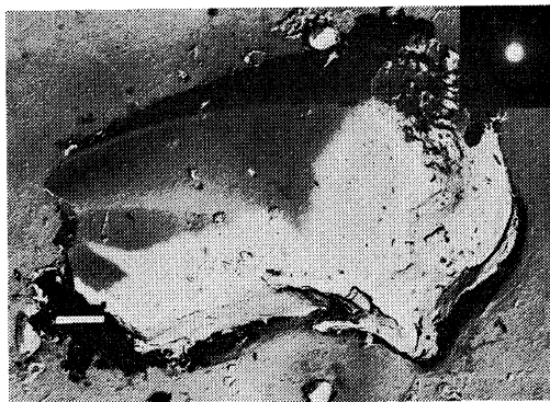
Figure 1. Electron micrograph of single crystal from the melt. Inset: electron diffraction pattern. Scale bar represents 1 \mu .
