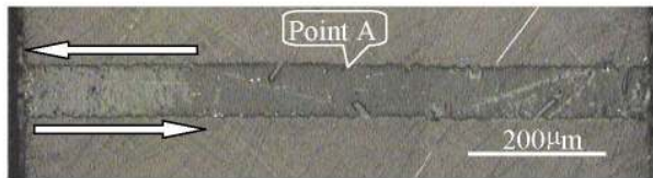
Fig. 9 PL image of a small Sn3.8Ag0.7Cu solder joint before mechanical tests. b = 100 \mu\text{m} . Arrows indicate the shearing loading direction.
