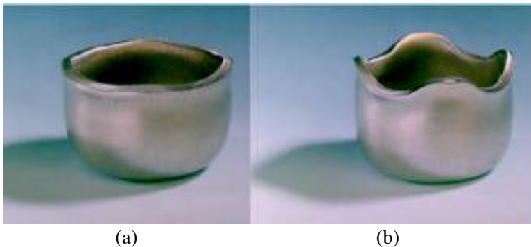
Figure 4: Aluminium cup (a) without ears, (b) with ears (courtesy Vaw Aluminium AG, Bonn).
