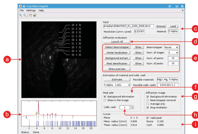
Figure 3 User interface of ringGUI . (a) Visualization of partial and final results in the input image; (b) visualization of assignment between measured peaks/rings (top) and theoretical d -spacing values (bottom); (c) input image details; (d) button launching the whole analysis; (e) buttons launching individual steps of the analysis procedure and basic settings; (f) settings of the peak plot; (g) instruments for enhancement of the input image; (h) calibration coefficient; (i) details about the peak/ d spacing selected in the peak plot.
