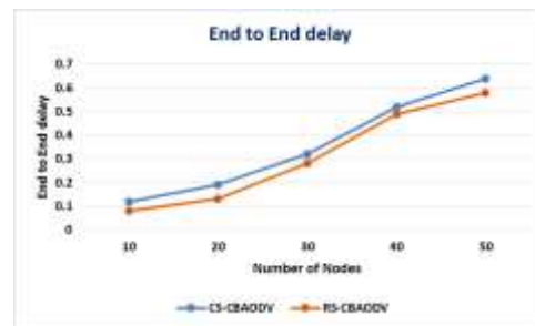
Fig.7. Comparison of End to End Delay by varying number of nodes
