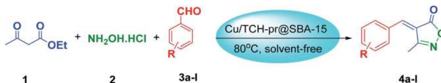
Scheme 1 The synthetic pathway of isoxazole-5(4H)-one derivatives.
