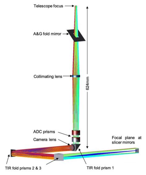
Fig. 4 3D optical scheme of the fore-optics sub-system of the CUBES instrument
