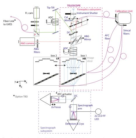
**Fig. 2** Functional scheme of the CUBES system (in which the light path goes from top to the bottom). The following acronyms are used: DC - dichroic, P - pinhole, Ps - series of pinholes, A&G - Acquisition and Guiding, AFC - Active Flexure Compensation system, FL - fiber link, ADC - Atmospheric Dispersion Corrector. Optional modules (TBD in Phase-B) are marked with a trefoil sign
