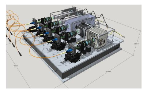
Fig. 9 3D mechanical concept for the lamp assembly of the calibration unit
