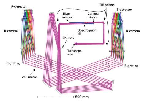
Fig. 3 Optical end-to-end model of the CUBES instrument
