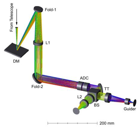
**Fig. 7** FiberLink FE module: A doublet (L1), placed behind Fold-1 and dichroic mirror (DM) collimates the beam, sending it through an ADC while passing a second fold mirror (Fold-2). A fast tip-tilt (TT) mirror, located in the pupil of L1, folds the optical path towards the camera (L2) which images the field at F/3 telecentrically onto the fiber tips
