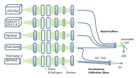
Fig. 8 Schematic concept of the calibration unit
