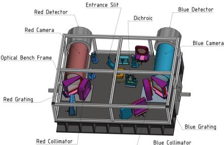
**Fig. 6** Mechanical concept for CUBES: The general layout of the main mechanical components is shown in the upper image. For reference, the Telescope Adapter has a diameter of about 1.5 m. The Fore-Optics Assembly is located near the center of the bench, while the spectrograph opto-mechanics are 'hanging' on the bottom side of the same bench (lower image)
