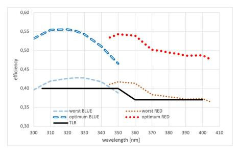
**Fig. 11** Calculated detective quantum efficiency of the two arms of CUBES (BLUE and RED) for *worst* and *optimum* scenarios. The black line indicates the formal top-level efficiency requirement. The throughput was calculated from the telescope focus, including detector QE, IS vignetting, but excluding atmospheric effects and telescope losses
