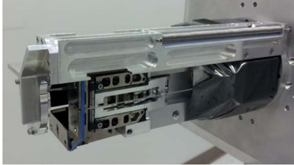
Figure 2: Deployable Petal Telescope in the Stowed Configuration
