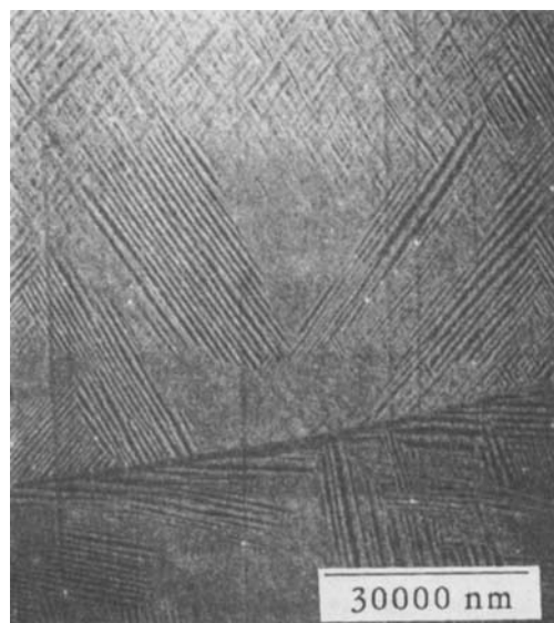
Fig. 2. A 6.0 mol% \text{Y}_2\text{O}_3 arc-melted sample containing several orientations of t' phase.
