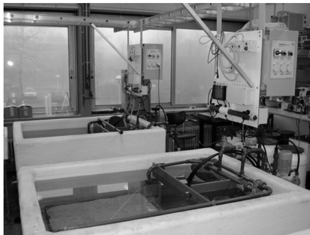
Fig. 3: Example of two ex situ cultivation tanks (1.3 m 3 ), in which water quality can be continuously measured and controlled, at Wageningen University.
